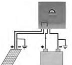
Be aware that the 50 Amp Pro Series Charge Controller is negative grounding and the negative terminals of the 50 Amp Pro Series Charge Controller are connected internally and therefore have the same electrical potential. If any grounding is required, always do this on the negative wires
