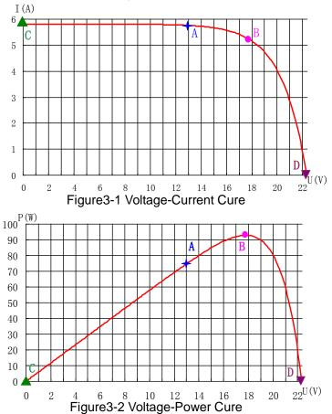
MPPT means maximum power point tracking. It makes the solar panels work at maximum point(ext Point B) by using power conversion technology. eMPPT is the new charge controller researched and developed by our company, and it uses the MCU to track the maximum power point of solar panels intelligently to generate more power from the solar panels.
