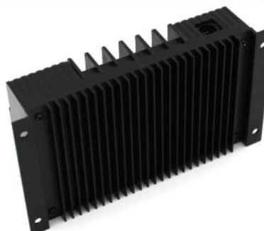
SR-LM2420 Dimension as below Overall dimension : 154×72×32.7(mm) Installation dimension : 144×50(mm) Installation hole diameter : 4.5(mm)
