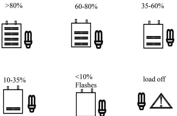
Pushing button within one second, load will manually on or off.
