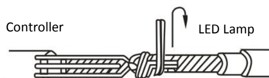
Figure 2.4.2 Second step during wiring - connection
