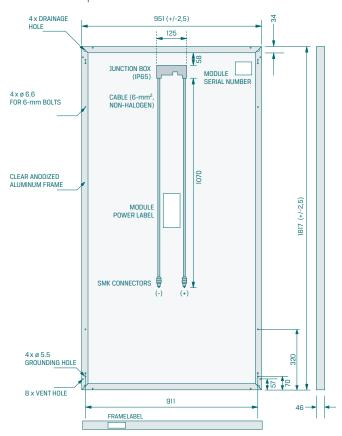
All dimensions in mm; module weight 20.1 kg
