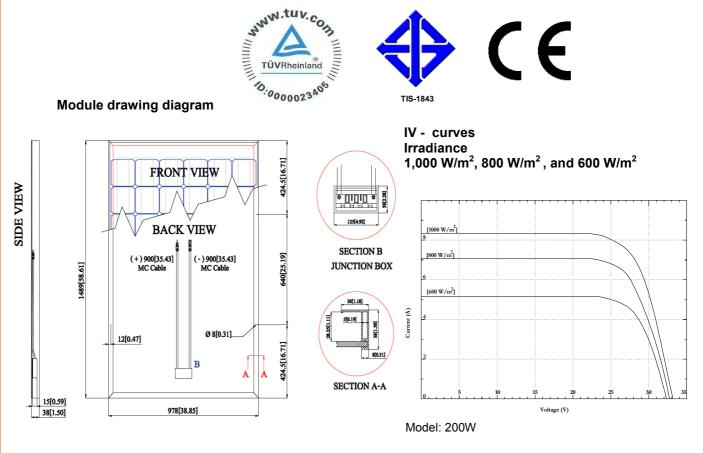
These data represent the performance of typical modules as measured at their out put terminals, and do not include the effect of such additional equipment as diodes or cables. The data are based on measurements made in accordance with ASTME1036-85 corrected to SRC (Standard Reporting Conditions, also known as STC or Standard Test Conditions), which are:
