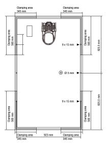
Module dimensions (L  $\times$  W  $\times$  H): <sup>1</sup>  $1,651 \times 986 \times 46 \,\text{mm}$ Cell dimensions: 156 × 156 mm No. of cells:
