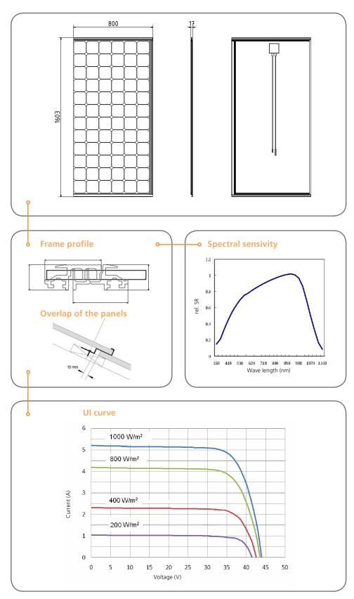
\*Standardized measures (STC), radiation:1000W/m², cell temperature: 25°C, AM 1 5
