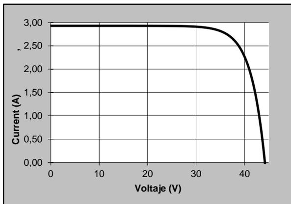
The electrical specifications are under test conditions of irradiance of 1 kW/m<sup>2</sup>, Spectrum of 1.5 air mass and cell temperature of 25°C.
