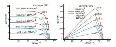
STC: Irradiance 1000W/m<sup>2</sup>, Module temperature 25°C, AM1, 5 spectrum
