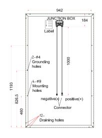
Dimension: 1653mm x 992mm x 40mm (46mm) Cells: 60 polycrystalline 156x156mm cells
