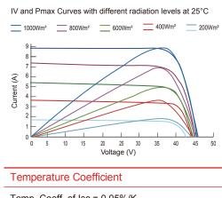
Temp. Coeff. of lsc = 0.05%/K Temp. Coeff. of Voc = -0.33%/K Temp. Coeff. of Pmax = -0.47%/K
