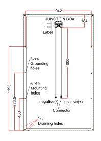
Dimension: 1653mm x 992mm x 40mm (46mm) Cells: 60 mono-crystalline 156x156mm cells Connection: Junction box IP65 with 3 bypass diodes Cable: 4mm2x1.0m with Tyco or MC4 compatible
