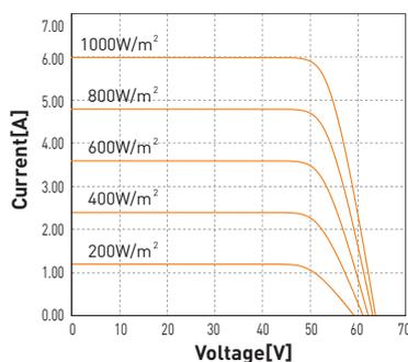
Reference data for model VBHN294SJ45(Cell temperature 25°C)
