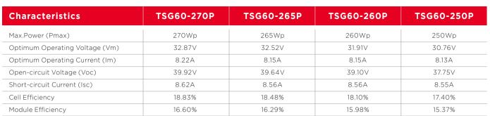
\*STC (Standard Test Condition): Irradiance 1000W/m<sup>2</sup>, Module Temperature 25°C, AM=1.5. \*NOCT: Irradiance 800W/m<sup>2</sup>, ambient Temperature 20°C, wind speed 1m/s.
