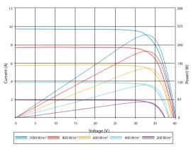
Excellent performance under weak light conditions: at an irradiation intensity of 200 W/m<sup>2</sup> (AM 1.5, 25 °C), **96.5%** efficiency (200 W/m<sup>2</sup>) is achieved
