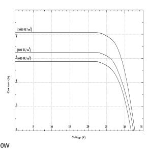
These data represent the performance of typical modules as measured at their out put terminals, and do not include the effect of such additional equipment as diodes or cables. The data are based on measurements made in accordance with ASTME1036-85 corrected to SRC (Standard Reporting Conditions, also known as STC or Standard Test Conditions), which are:
