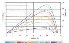
Current-Voltage & Power-Voltage Curves At Different Irradiances
