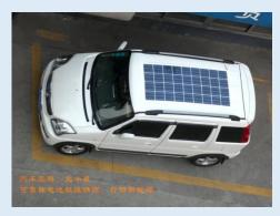
弯曲板应用于改装车,和应用于房车有同等效果。弯曲板重量轻,安装可贴合车顶弧面,美观实用。 The bending plate is applied to the reloading vehicle, which has the same effect as the motor vehicle. The bending plate weighs light, the installation can be fitted with the roof arc, beautiful and practical.
