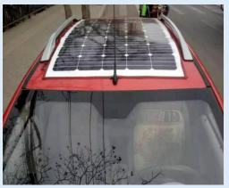
低速城用电动车安装太阳能电池板后,太阳能电池板为车载动力电池供电,延长行驶里程,保护电瓶。After the low-speed city USES electric cars to install solar panels, the solar panels provide power to the car's power battery, extend the mileage and protect the battery.
