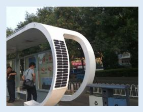
公交站的 LED 灯采用太阳能供电会节省很多维护成本。太阳能供电系统采用弯曲组件供电,造型美观,适用于现代化城市建设。The use of solar power by the LED lights of the bus station will save many maintenance costs. The solar power supply system USES curved components to power supply, beautiful shape, suitable for modern city construction.
