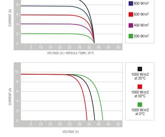
\*STC: (Standard Test Condition) Irradiance 1000W/m²; Module Temperature 25°C; Air Mass 1.5
