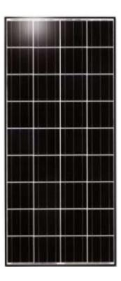
The SPA 230 photo voltaic Solar Panel is a Zone 2 ATEX Ex nAnC certified product for hazardous area applications. The cells of the panel are encapsulated between a tempered glass cover and are EVA pottant - to provide maximum protection in the most extreme environmental conditions.
