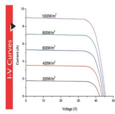
\* Irradiance of 1000W/m , spectrum AM of 1.5 and cell temperature of 25°C
