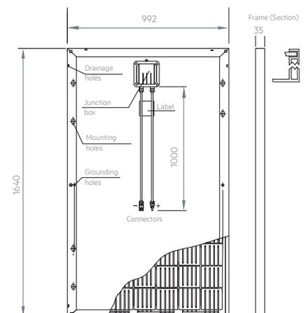
Module dimensions in the technical picture are expressed in mm with tolerance ±2 mm (±0.079 ")
