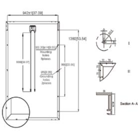
Dimensions in brackets are in inches. Un-bracketed dimensions are in millimeters. Unit: mm[in.]
