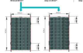
\*\*Installation with Alumero fixing clamps END/MID 6.8 100 mm allowed only for landscape orientation configuration.
