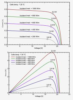
STC: Irradiance 1000W/m<sup>2</sup>,Module temperature 25°C, AM1.5 spectrum.
