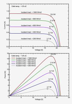
STC: Irradiance 1000W/m<sup>2</sup>,Module temperature 25°C, AM1.5 spectrum.
