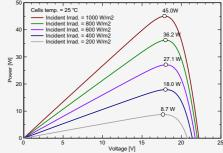
STC: Irradiance 1000W/m<sup>2</sup>,Module temperature 25°C, AM1.5 spectrum.
