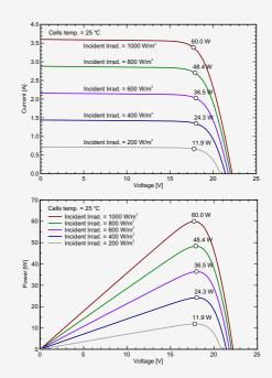
STC: Irradiance 1000W/m<sup>2</sup>,Module temperature 25°C,AM1.5 spectrum.
