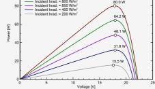
STC: Irradiance 1000W/m <sup>2</sup>,Module temperature 25°C,AM1.5 spectrum.
