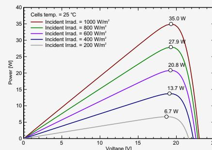
STC: Irradiance 1000W/m<sup>2</sup>, Module temperature 25 $^{\circ}$ C, AM1.5 spectrum.
