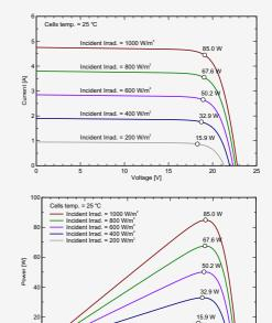
STC: Irradiance 1000W/m<sup>2</sup>,Module temperature 25°C,AM1.5 spectrum.
