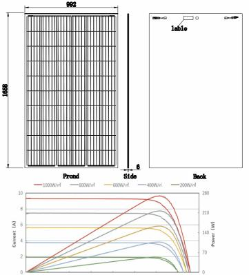
$\label{eq:Voltage_Voltage} \begin{tabular}{ll} Voltage (V) \\ Excellent performance at 200W/m^2(AM 1.5, 25 C°): the conversion efficiency could be 96.2% of STC. \end{tabular}$
