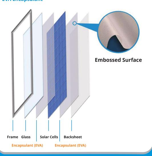
'CONSERV A 360 - 10 UC' is an Ultra-fast cure, UV and weather stable Ethyl Vinyl Acetate (EVA) PV Encapsulant, proven for single stage as well as short cycle multi stage lamination processes. This Encapsulant can be used for all Crystalline and many Thin - Film PV Modules. It has standard UV cut off wavelength.
