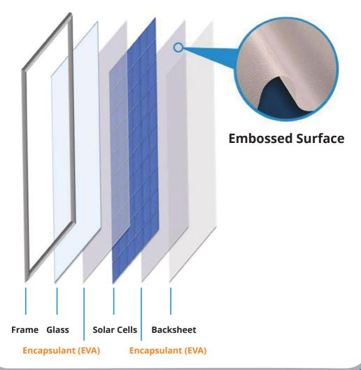
'CONSERV P UVT - 14 FC' is a wide process window curable, PID resistant, UV and weather stable Ethyl Vinyl Acetate (EVA) PV Encapsulant, proven for single stage as well as short cycle multi stage lamination processes. This Encapsulant is specially recommended for PV Crystalline Modules used in tropical (Hot and Humid) climatic conditions. It allows PV Modules comprising blue-light sensitive cells of a given efficiency, to generate higher power.
