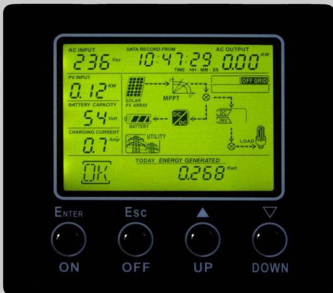
Above: All the important data of your PV system can be monitored via the extensive display.
