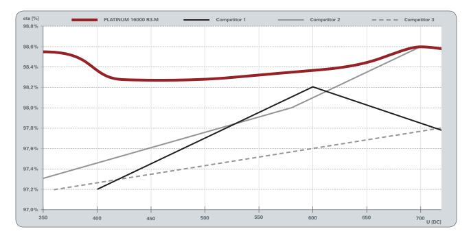
High efficiency across the entire MPPT voltage range thanks to innovative Dual- $X^{\circ}$  technology. The advantage: exceptionally high yields with optimum design flexibility.
