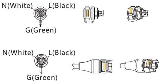
**Step4** Plug the AC output line to main AC cable;
