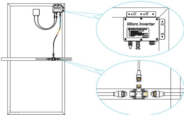
**Step2** Connect the two DC terminal of the PV to the inverter, positive to positive, negative to negative. Show below:
