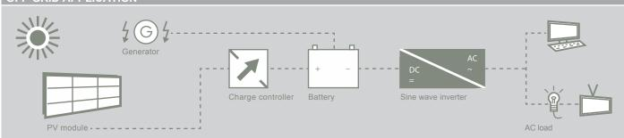
The inverter converts the DC battery voltage (direct current) into  $230V_{AC}$  (sinusoidal alternating current). Voltage-controlled, it provides a stabilized, quartz-precise direct current of  $230V_{AC}$ /50Hz (other voltages and frequencies as per type label). All conventional consumption items such as energy-saving light bulbs, computers, engines, pumps, radio and HiFi systems can be operated with the sinusoidal inverter.
