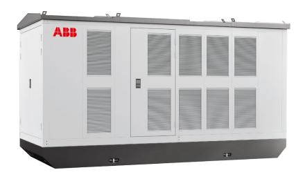
The ABB medium voltage housing is a plug-and-play solution designed for large-scale solar power generation and to be compatible with the PVS800 inverter station. It houses the medium voltage transformer and the switchgear equipment needed to rapidly install and connect the inverters to the medium voltage network of the photovoltaic plant.
