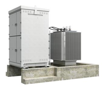
The ABB medium voltage pad mounted solution is a cost efficient and robust solution designed for large-scale solar power generation and to be compatible with the PVS800 inverter station. It combines the medium voltage transformer and the switchgear equipment needed to connect the inverters to the medium voltage network of the photovoltaic plant.
