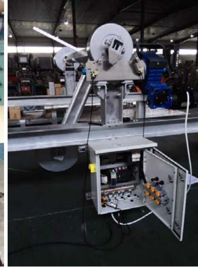
Lifetime test: Main components reliability test ; Include : Load、 impact load、 accelerated aging , high-low temperature test、 IP grade、 UV.
