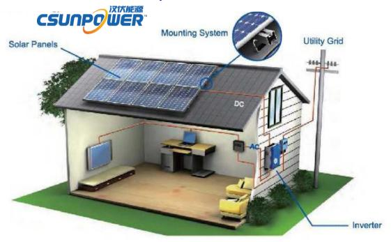
On grid solar system is a renewable energy system, which can transfer solar energy into electricity and inject it to power grid. The energy generated from solar system will offset the energy customer used from power grid, so as to help reduce cost of monthly electricity bill, and enjoy life with clean energy.
