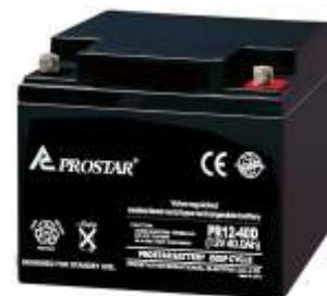
PR12-40D is AGM Deep cycle battery with 10 years floating design life, specially designed for frequent cyclic discharge usage. By using strong grid and specific paste plate, it makes battery have 30% more cyclic life time than standby series. It is applicable for solar energy system, golf cart, electric wheelchair, etc..
