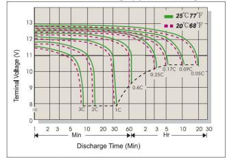
Discharge Current VS. Discharge Voltage
