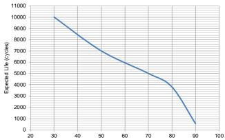
XNote: It is time to replace all batteries when the batteries reach the expected life (cycles) or the maximum length of use (15 years), whichever comes first.
