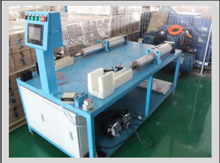
Solar Mounting System Push Testing Machine
