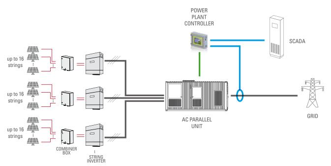
Our products for photovoltaic industry, highly advanced technologically, then complete FIMER's range of offerings. The new 3PH R series string inverters have been specifically designed for mainly commercial and large scale distributed PV Plants both indoor and outdoor (IP 65).
