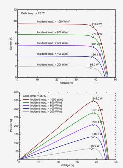
STC: Irradiance 1000W/m<sup>2</sup>,Module temperature 25°C,AM1.5 spectrum.
